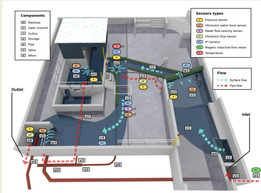
Figure 1: Overview of the floodable area of the floodX flood facility, illustrating main hydraulic flows on the surface (blue arrows), and in pipes (red arrows). The labels indicate major hydraulic components and the placement of sensors, with the IPC labels indicating what component is in the centre of each camera view.
