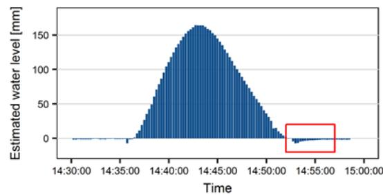
**Figure 4:** Measured water level in basement s6 by ultrasonic sensor s3\_h\_us\_maxbotix presents abnormally low values after flooding (negative water levels of up to -7 mm can be seen in the red rectangle).
