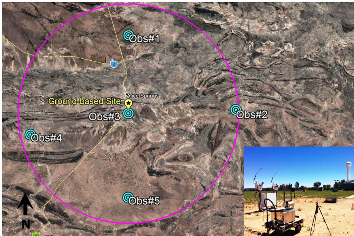
**Figure 3.** A Google Earth map showing the GOSAT specific point observations around Alice Springs (cyan circles labeled "Obs#") . The ground-based site is securely fenced and located at the airport, c. 14 km south of the town center. The magenta circle shows a 60-km radius from the site, for visual reference. The inset shows the EM27 during the measurements.
