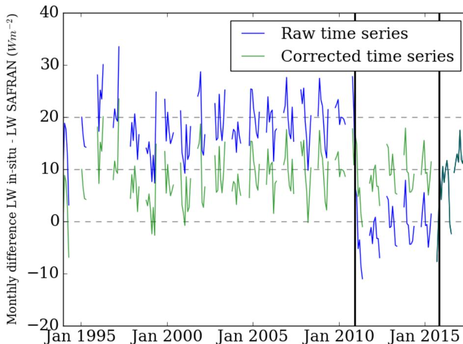
**Figure 5.** Monthly average of the difference between measured downward longwave and SAFRAN estimates. The two vertical black lines indicate the sensor changes (cf Table 2). The blue lines correspond to the raw time series and the green one to the corrected time series.
