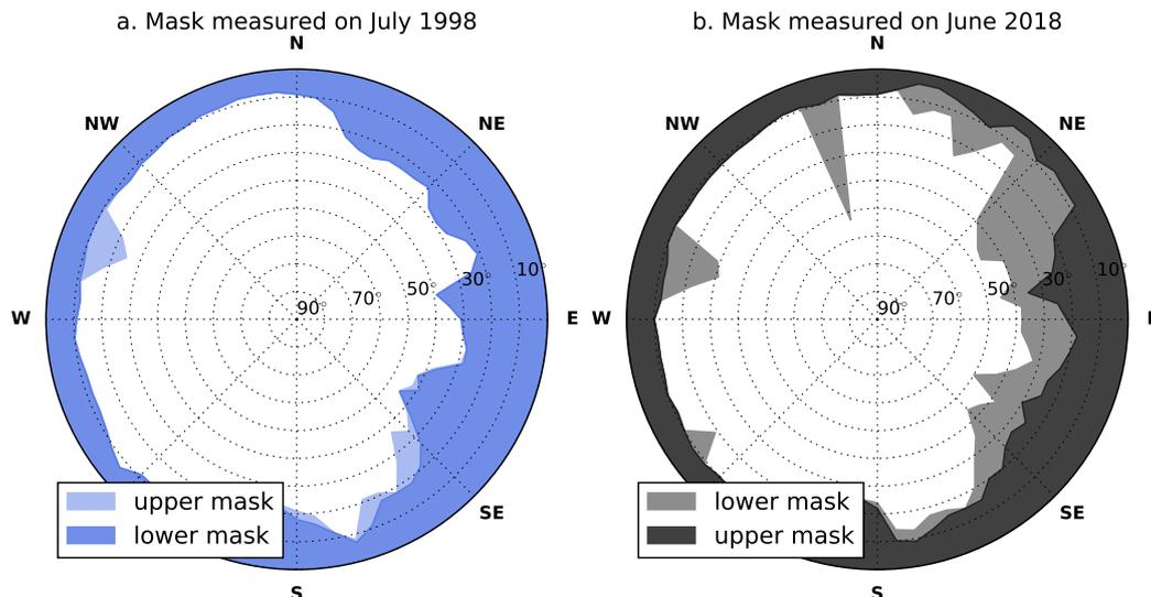
**Figure 3.** Masks measured at location 31 on July 1998 (left panel) and on June 2018 (right panel). Upper and lower mask elevations are represented by the coloured areas. Elevations are given in degrees, the center is 60 degrees elevation.
