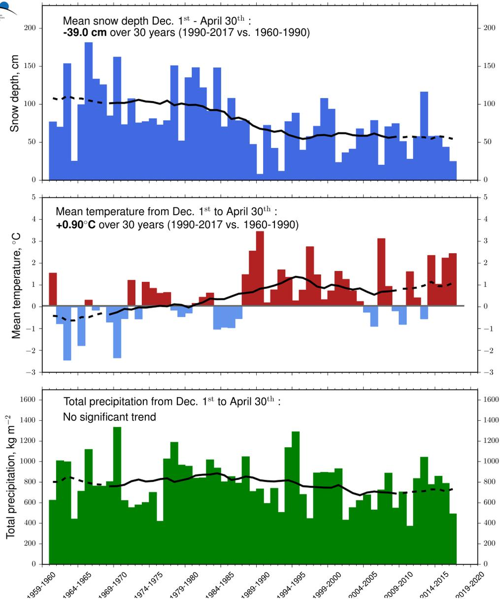
**Figure 11.** Evolution of mean snow depth, air temperature and total precipitation over 1960-2017. The mean and total values are calculated over the period 1 December to 30 April of each snow season. The black lines are 15-year moving means.
