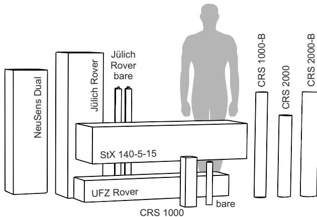
**Figure 2.** Dimension of CRNS sensors employed in the campaign. The blocks illustrate the size of the detectors; the actual units also comprise other components, combined in a slightly larger housing.
