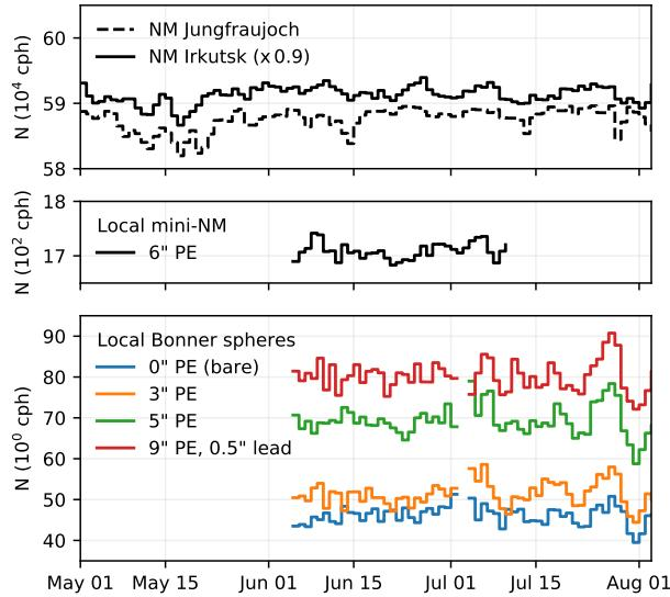
**Figure 5.** Neutron count rate  $N$  for different detector types: the remote neutron monitors at Jungfraujoch and Irkutsk, the local Mini-NM, and the local Bonner Spheres. Each instrument is equipped with different PE or lead shields to adjust the detection sensitivity towards different neutron energies.
