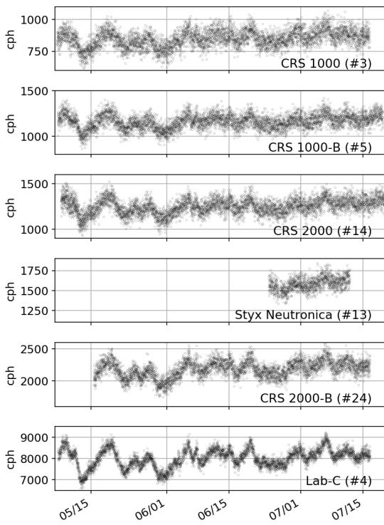
**Figure 3.** Raw (not standardized, uncorrected) neutron count rates (in counts per hour, cph) recorded at an integration interval of 20 minutes by six exemplary CRNS sensors representing different manufacturers/models (sensor ID in parentheses, see Tab. 2). While the qualitative dynamics are visually similar, the different sensitivities become evident by both different averages and different signal-to-noise ratios - please mind the different y-axis scaling.
